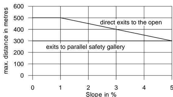
**Figure 2:** Distance of emergency exits as a function of slope for bi-directional tunnels according to [6]
