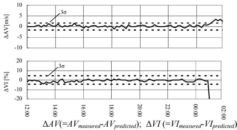
**Figure 2:** Sensor failure at approximately 01:00 hours
