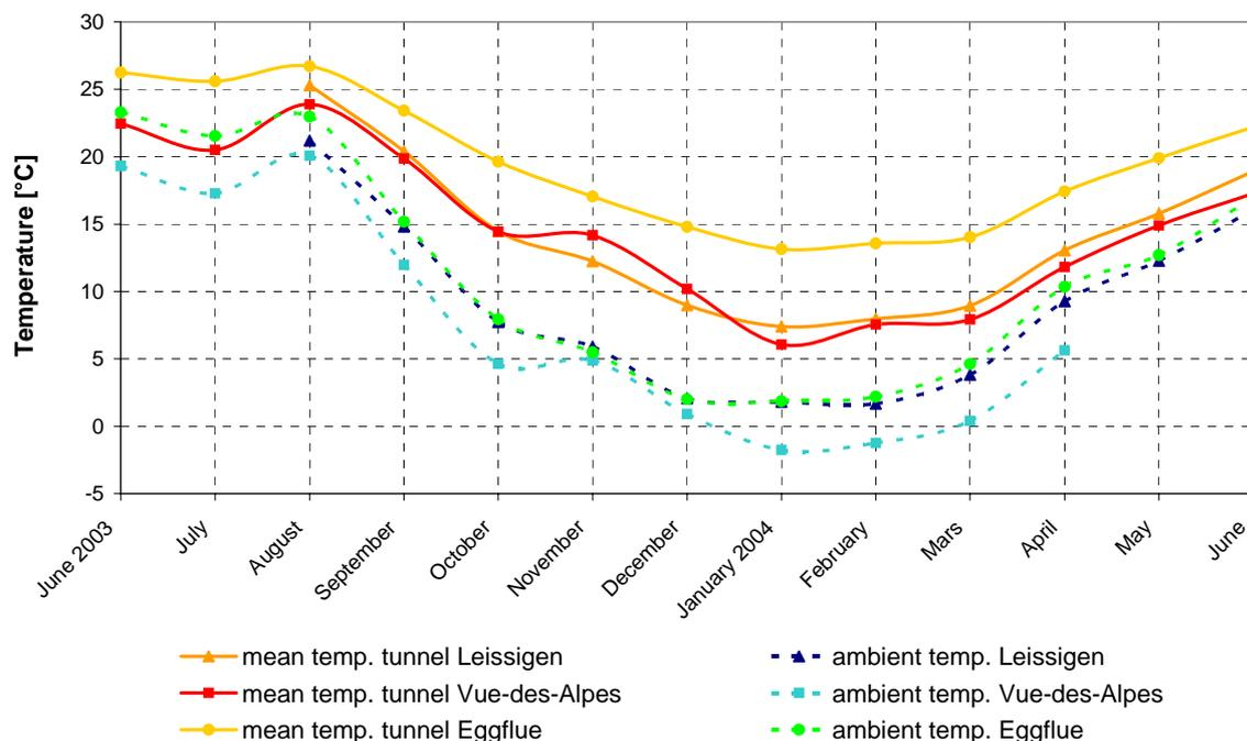
**Figure 3:** Monthly mean temperatures (ambient and tunnel) for Leissigen, Vue des Alpes, Eggflue<sup>1</sup>. Period: July 2003 to June 2004.
