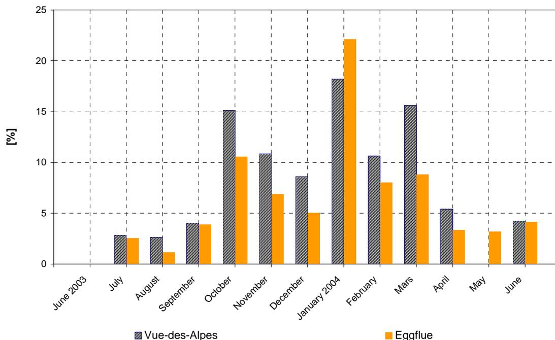
**Figure 4:** Time slices during which windshield fogging has to be expected based on measured data and a threshold value of  $1.5 \text{ g/m}^3$  (Vue-des-Alpes and Eggflue). Period: July 2003 to June 2004.
