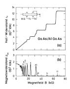
Figure 2: Results of the measurements of the Quantum-Hall-resistivity (a) and the Shubnikov-de Haas-oscillations [2]
