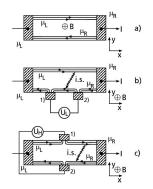
Figure 1: a) electron transport in the edge-channels of a 2DEG, b) measurement of the resistivity parallel to the current (Shubnikov-de Haas oscillations), c) measurement of the Quantum-Hall-resistivity [1]
