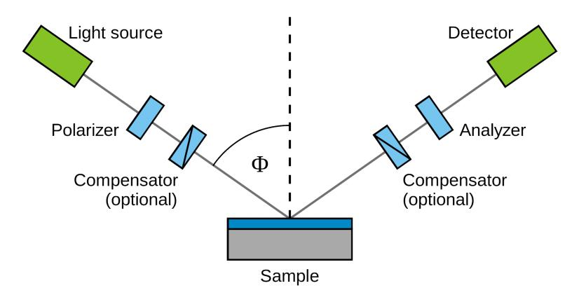
Ellipsometry measures the change of polarization upon reflection. The measured signal depends on the thickness and the dielectric constant.
