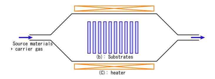
Epitaxial silicon CVD SiH<sub>4</sub> (silane) or SiH<sub>2</sub>Cl<sub>2</sub> (dichlorosilane) PH<sub>3</sub> (phosphine) for n-doping or B<sub>2</sub>H<sub>6</sub> (diborane) for p-doping.
