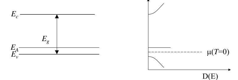
p-type:  $p \sim N_A$  Many more holes in the valence band than electrons in the conduction band.
