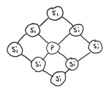
Easier to ionize a P atom in Si than a free P atom
