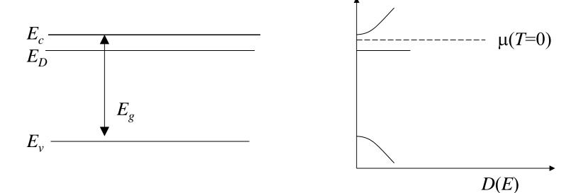
n-type:  $n \sim N_D$  Many more electrons in the conduction band than holes in the valence band.
