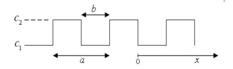
The dielectric constant and speed of light are different for the two layers.
