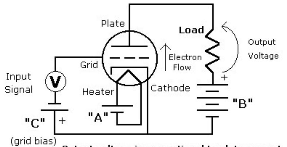
Output voltage is proportional to plate current, which is controlled by grid voltage.
