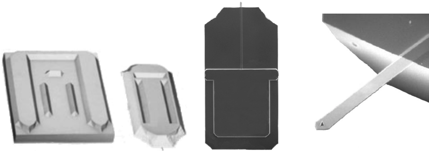
Figure 3-1: Cantilever. (Left) Alignment system. (Center) Cantilever chip viewed from the top. (Right) Cantilever, 450 \mu\text{m} long, 50 \mu\text{m} wide with integrated tip.
