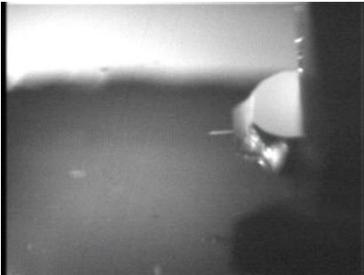
Figure 4-1: View of the cantilever after coarse approach.
