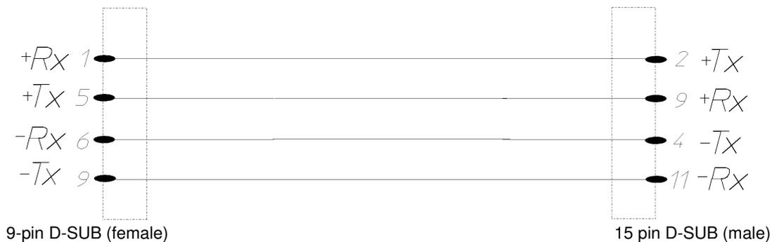
*Pin assignment for RS 485 interface cable for Anaprog controllers*
