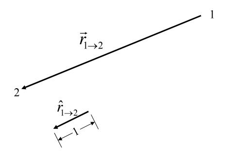
$$\hat{r}_{1\to 2} = \frac{\vec{r}_{1\to 2}}{|\vec{r}_{1\to 2}|} = \frac{(r_{2x} - r_{1x})\hat{x} + (r_{2y} - r_{1y})\hat{y} + (r_{2z} - r_{1z})\hat{z}}{\sqrt{(r_{2x} - r_{1x})^2 + (r_{2y} - r_{1y})^2 + (r_{2z} - r_{1z})^2}}$$
