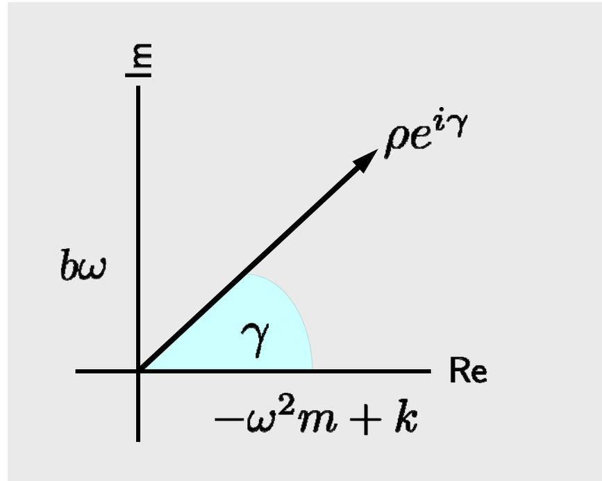
$$\tan \gamma = \frac{b\omega}{m\left(\frac{k}{m} - \omega^2\right)} = \frac{b\omega}{m(\omega_0^2 - \omega^2)}$$
