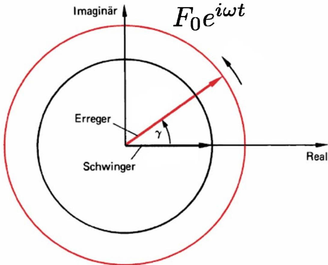
$$z(t) = \frac{F_0}{\sqrt{b^2 \omega^2 + (k - m\omega^2)^2}} e^{-i\gamma} e^{i\omega t}$$
