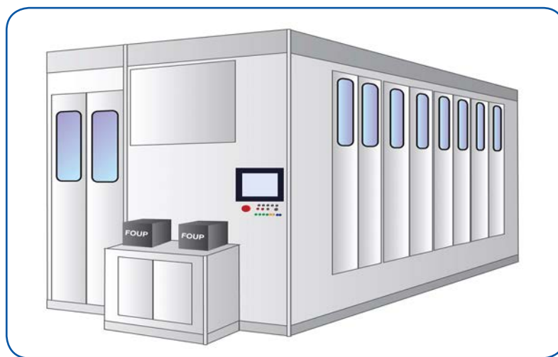
Figure 111. A modern wet bench cleaning station [191].
