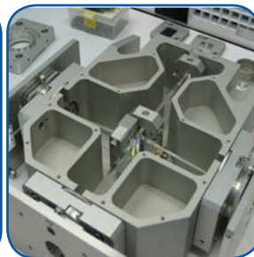
Figure 215. High power LED illuminator for use in inspection tools.
